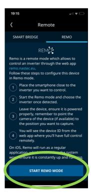
Select the Nastec device nearby to be controlled (in the device verify that BTLE parameter is set to ON).
