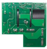
In traditional boosters the starting relay is triggered by the voltage value across the starting coil which disconnects the starting capacitor after the motor has started. The limitations of this system are that different relay models are required depending on the motor used, supply frequency, maximum voltage of the starting coil and the on/off voltage of the starting capacitor. IThis requires a large stock of voltage relays specific to each motor and each manufacturer.
